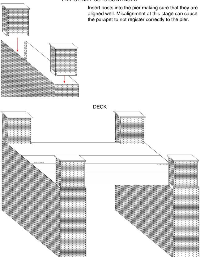
Glue the first deck element to the piers thus joining two piers together. The deck was designed to be a very close fit and it is normal for it to be slightly reluctant to locate in place. Apply gentle force to push the second deck element into place but be careful not to strip bricks off the posts. If the deck is too tight trim off some material from the inner seam.
